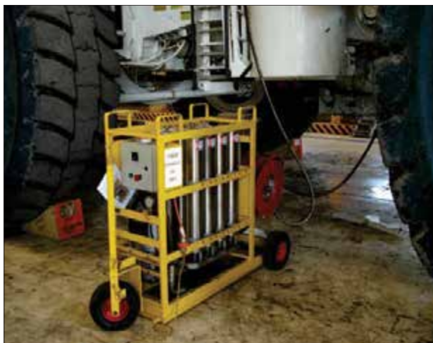
FM60842 filtering hydraulic oil on a Komatsu 830E
