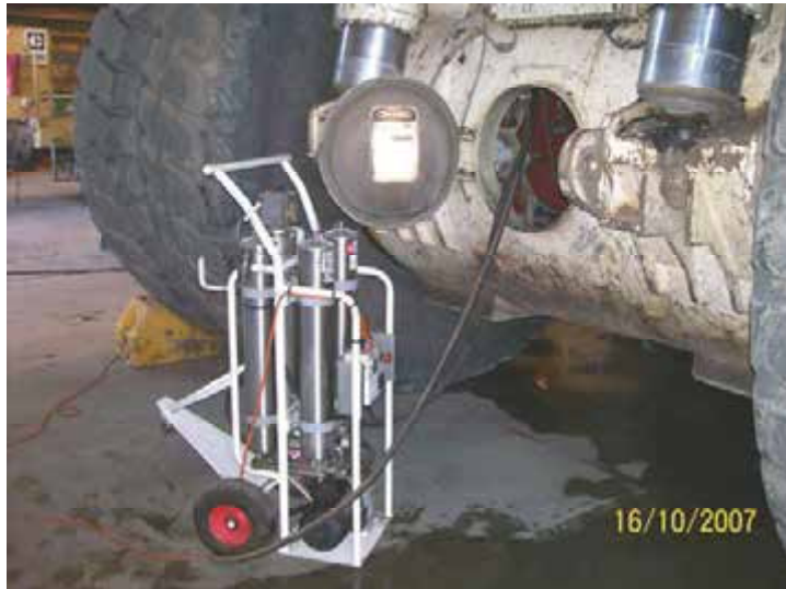
Kidney filter cart with heater designed to suit 680 grade oil for GE wheel motors
