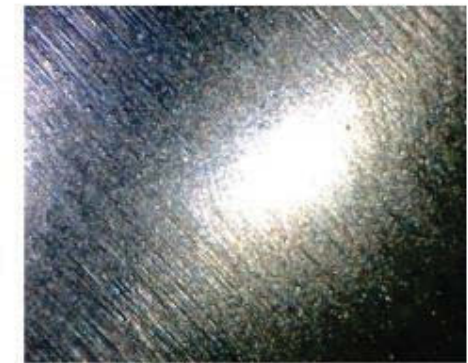
793C Final Drive Wheel Bearings @ 18,000 SMU 4000 Hour Oil Change Intervals "With Kidney Looping"
