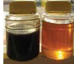
Oil before and after filtration
