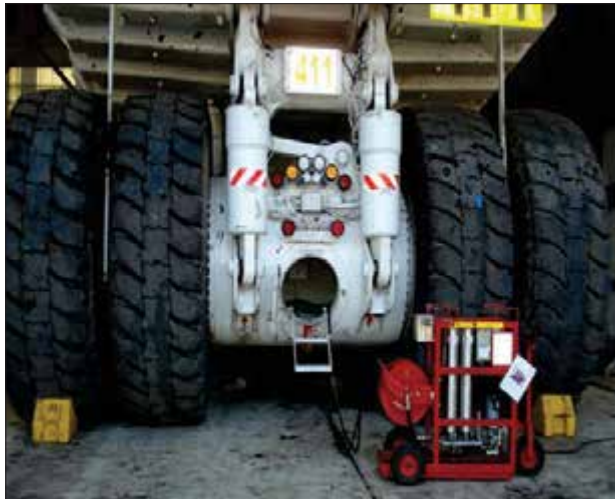
FM60442 filtering wheel motor oil on a Komatsu 830E
