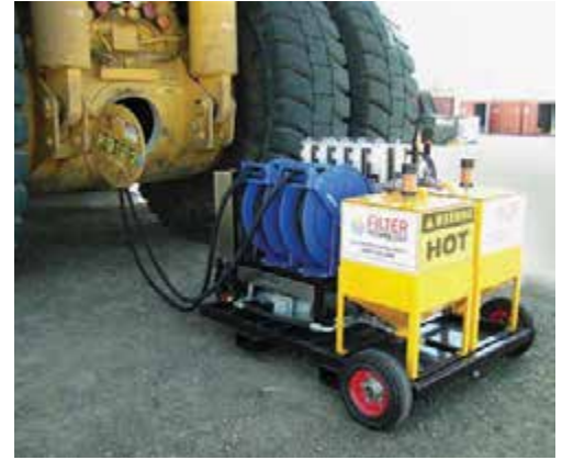
Kidney loop filtration on final drive unit using mobile filtration buggy
